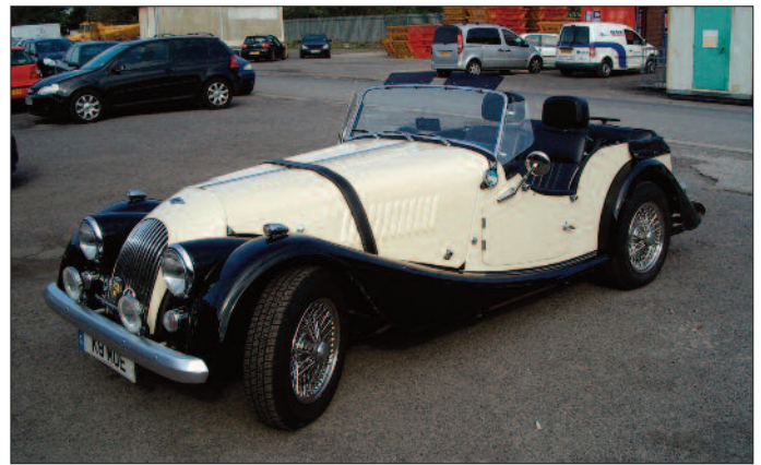
Martin & Vivien Cocks. 1st re-build. 1992 4/4 4 Seater. Ford 1600 cvh injection as fitted to the XR2.
