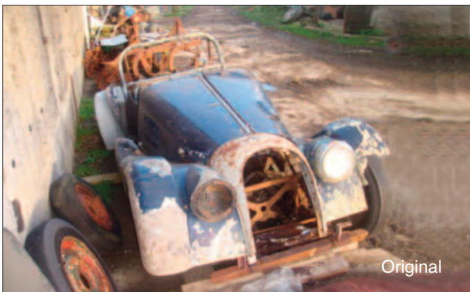
Martin & Vivien Cocks. 3rd re-build. 1956 4/4. Ford 1175 upgraded to a 1500 Ford Cortina GT.
