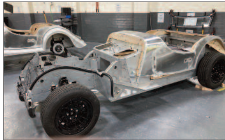
Peter and Rosemary meet the man working on the build, with work on the chassis and fitting of the aluminium body panels.
