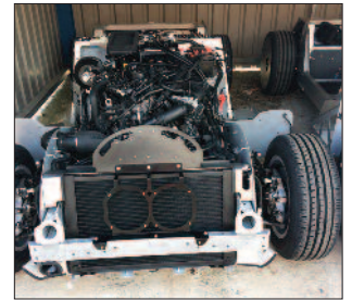
The order details for continuing the build, with rolling chassis completed, engine and gearbox prepared and fitted to the chassis.
