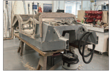
The chassis delivery, before Peter and Rosemary attend to see the build in progress, which commenced fitting the Ash frame.
