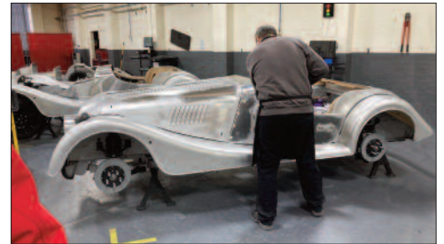
Peter and Rosemary meet the man working on the build, with work on the chassis and fitting of the aluminium body panels.
