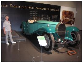
This a Bugatti Royale Esders, claimed to be the largest car in the world. Weighing in at over 3 tonnes and with a 12.7 ltr straight eight engine it maybe. But that large engine only produced 270 bhp. Was that good in 1927?
