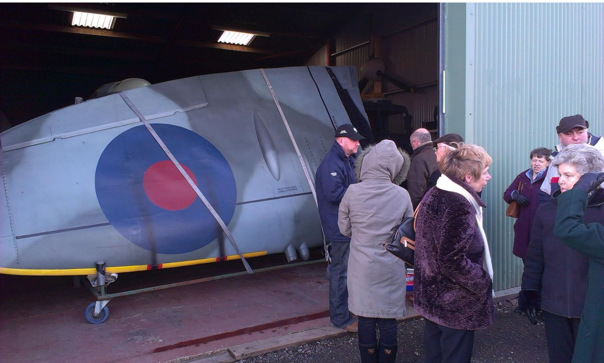
Detached wings on trolley waiting to be moved
